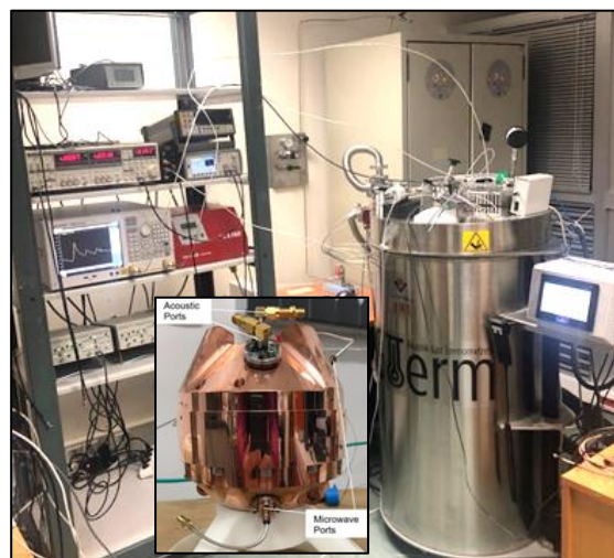
Figure 2. Primary acoustic gas thermometer (AGT) being developed by Tubitak for thermodynamic temperature measurements between 234 K and 303 K.
