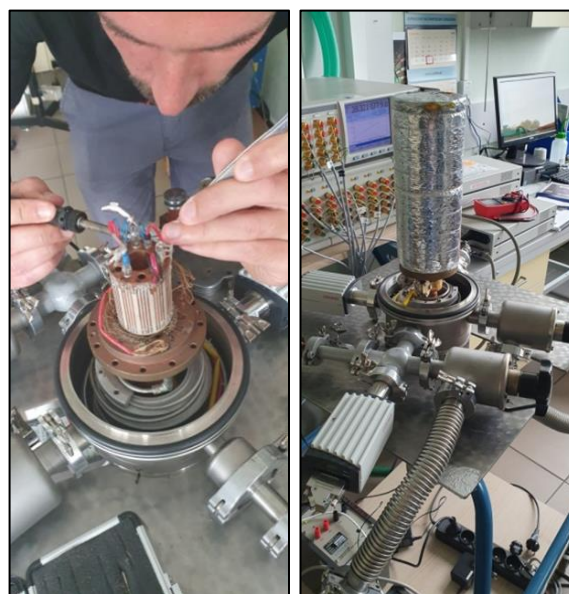
Figure 1. Cryogenic measurement system of INTiBS for ITS-90 calibration of capsule-type resistance thermometers between 9 K and 25 K.
